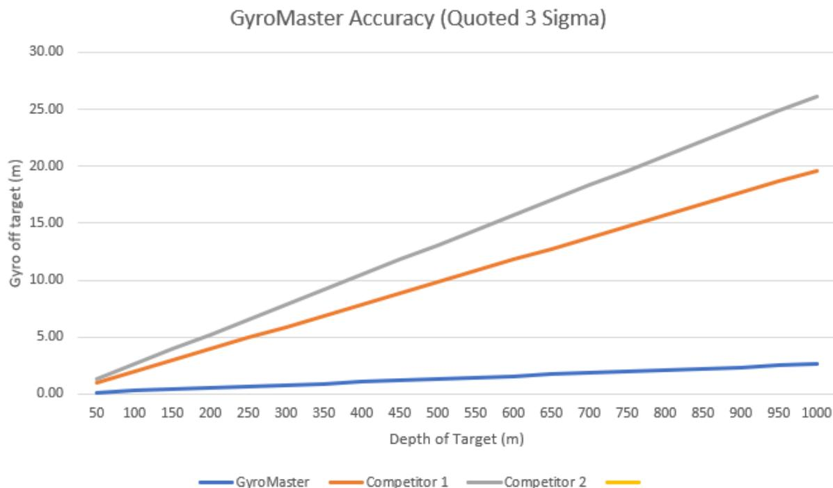
Figure 3. Accuracy of the GyroMaster™, comparing with other tools in the market
